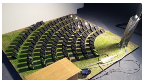
Figure 2. Model of a concentrated solar power plant (CSP)
