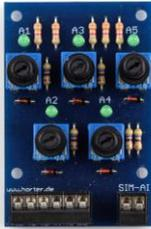
Fig. 7. Simulator for 5 analogue inputs
