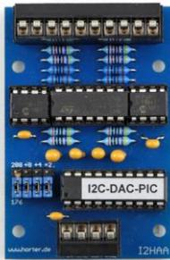
Fig. 6. Analogue output card 12 bit
