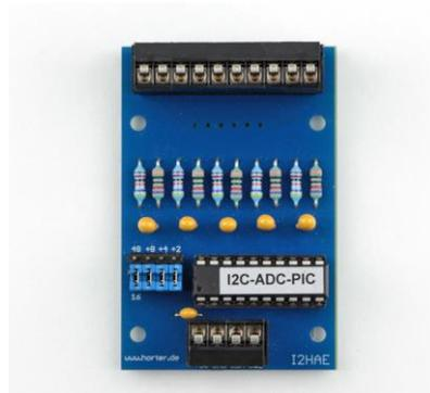
Fig. 5. Analogue input card 12 bit
