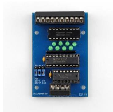
Fig. 4. Digital output card 8 bit
