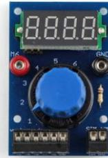
Fig. 8. Simulator for 6 different analogue values
