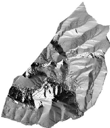
Fig. 5. Slope orientation for Ermua, from LIDAR data
