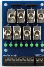
Fig. 9. Simulator for 8 digital inputs
