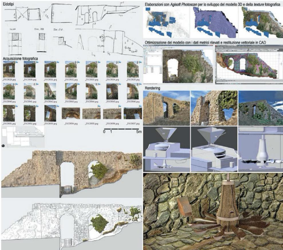
Fig. 6. Photogrammetric survey of the main adduction channel of the Olivo water mill and virtual reconstruction of the mechanism of a horizontal wheel mill.
