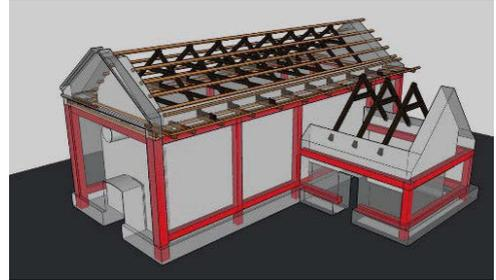
Fig. 4. Diagram of the reinforced concrete structure, in red, incorporated into the adobe walls in Uquía © Authors
