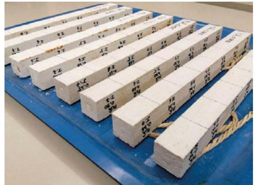
Fig. 2. Pieces of dimensions 290 x 25 x 25 mm
