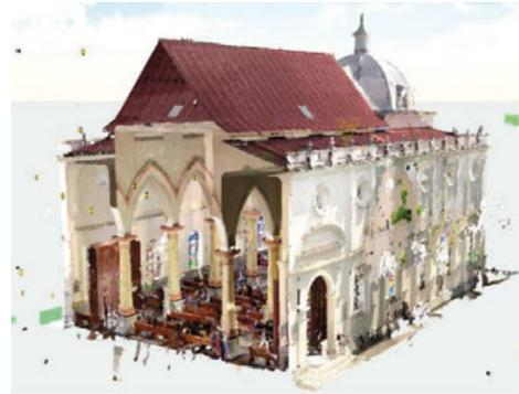
Fig. 4. Three-dimensional model by laser scanning. (Source: elaboration by Gómez Mejía, 2020).
