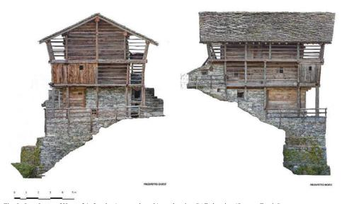
Fig. 8. Ortophotos of House 2 's facades (west and north) overlapping CAD drawing (Source: Frosini).
