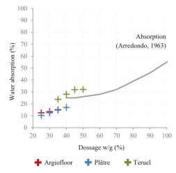
Fig. 9. Different water/gypsum dosage ratios vs water absorption
