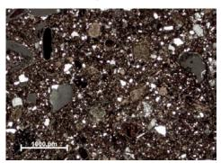
Fig. 14. Brick with an evident birifrengent groundmass and an abundant framework (image at the optical microscope in thin section, polarised light) (Source: Fratini).
