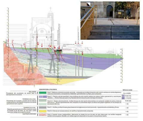
Fig. 3. Geotechnical correlation profile of all available information. (Source: Investigation report for the assessment of problems in the subsoil of the Juslibol church (Zaragoza), 2014). In the photograph it can be seen the crack number 4 recognisable in the square that is in front of the main door.
