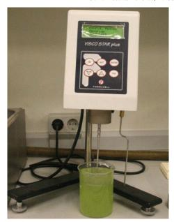
Fig. 1. Evaluation process of kinematic viscosity (η). (Source: Medina Lorente, 2022).
