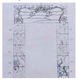
Fig. 7. Damage scheme. Chapel door. British Cemetery (Source: Benavent, 2017).
