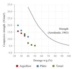
Fig. 8. Different water/gypsum dosage ratios vs compressive strength
