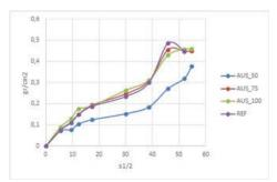
Fig. 6. Comparison of the results obtained in the test to determine the capillary water absorption of specimens made with *Austrocylindropuntia subulata* MUHLPFRDT and reference specimens.
