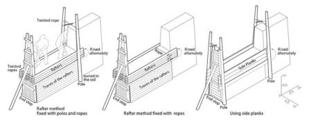
Fig.3. The segmented formworks (author)
