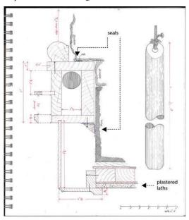
Fig. 2. Detail of the casing of a sash-window in a 19th century house in South Bend (IN-USA). The diagram shows the plastered laths employed to insulate the interior stone wall and horsehair and vegetable fibres to seal joints. (Source: Vitti)
