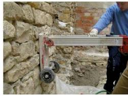
Fig. 6. Test about the internal composition of the façade of the Royal Butchers (16th century) in Porcuna, during the restoration process. It is possible to observe that the façade is charachterized by an orderly configuration, instead the "soul" of the wall is composed of filling material without any consistency. (Source: Millán, 2014).
