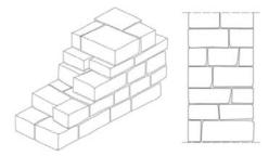
Fig. 6. Axonometric view and section of a M3 type masonry.
