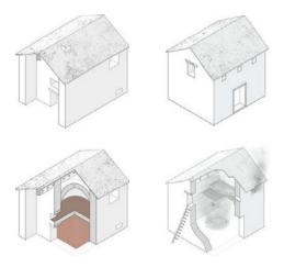
Fig. 3. Scheme of a oven (left) and a dryer (right) in Pratalec-
