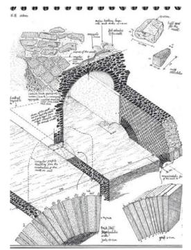
Fig. 4. Three-dimensional diagram analyzing the construction of the cistern of the Roman Villa at Capo Sorrento. The drawing shows materials, the way they were transformed and assembled. (Source: Vitti)
