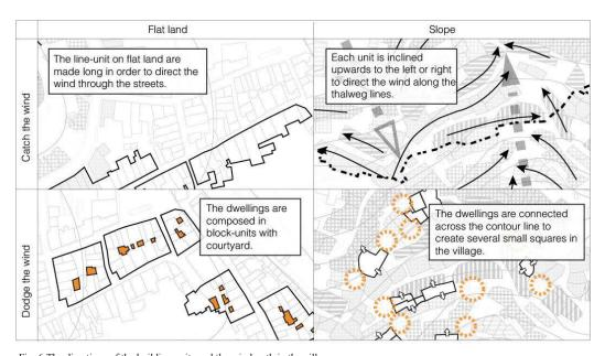
Fig. 6 The directions of the building units and the wind-path in the village
