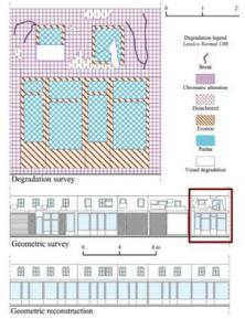
Fig. 11. Skopjie Bazaar: degradation survey and restoration of a commercial building (Source: Trematerra, 2022)
