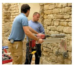
Fig. 7. Detail of the process of extracting the stone from a load-bearing wall to analyse its internal composition. It is possible to observe that the wall is without mortar but just a mud poor in lime. (Source: Millán, 2014).
