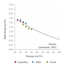
Fig. 6. Different water/gypsum dosage ratios vs bulk density
