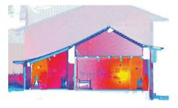
Fig. 7. Point-cloud image from the 3D database of Casa do Anhanguera in Brazil, highlighting the typical Portuguese colonial roof shape. The short digitization project involved local technicians and professionals to familiarize them with the technology and evaluate possible digital surveys on the most important vernacular buildings of the state of São Paulo (Image by the author).
