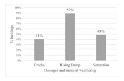
Fig. 5. Percentage of buildings with damages and material weathering.
