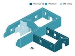
Fig. 11. Benevento, Acqualonga mill. Hypothesis of transformation (drawing by S. Cuntò, L. Intermoia, L. Longo, Restoration Studio, Dept. of Architecture, University of Naples Federico II, prof. V. Russo, July 2016).
