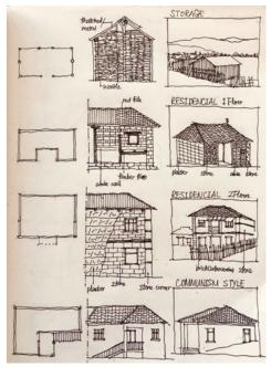
Fig. 5. Classification of local buildings "typologies" (Source: EHV, 2021).
