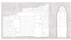
Fig. 6. Dry stone wall with boulders and shapeless stones (Source: Caleca, 2018)
