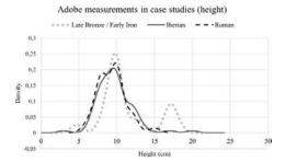
Fig 2. Most repeated dimensions according to Kernel density estimation of registered adobe (Source: S. Manzano Fernández, 2022).
