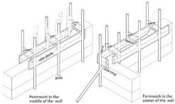
Fig.13 The formworks used in Jianchuan (author)
