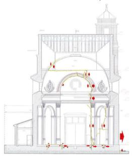
Fig. 5. Schematic profile of the main cracks and fissures that can be seen inside the church. The position and magnitude of the arrows express the apparent movement that the recognized deformation has developed. In the photograph, you can recognize some of the cracks in the part of the altar-presbytery.
