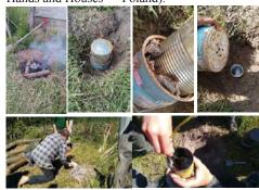
Fig. 2. [a, b, c, d, e & f]. Preparing a waterproofing additive for plasters from the bark of birch trees - Poland (2015).
