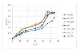
Fig. 7. Results obtained in the test to determine the water absorption by capillary action of the tested groups.
