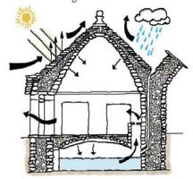
Fig. 7. Bioclimatic characteristics of a trullo (Drawing by the author, 2022).
