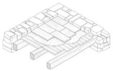
Fig. 4. Axonometric view of a single-joisted floor.
