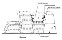
Fig. 6. Diagram of forces favoring transverse restraint in walls (Source: Torres, 2021).
