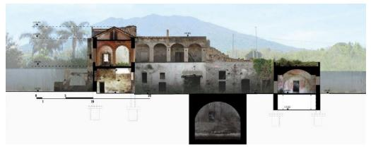
Fig. 4. A section on the courtyard of the masseria of the Duke of Salza. The section intercepts the cistern, along the shorter side, the room on the groundfloor where there was the scalandrone, a stable with the upper terrace, the meeting hall in the apartment of the administrator and the attic. On the background, there's the loggia facing the courtyard (Source: Author, 2018).
