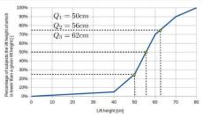
Fig. 8: Statistical analysis of wall height and lift height for the different cob buildings
