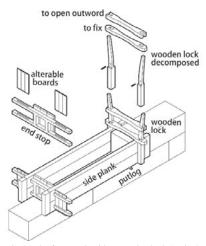
Fig.11 The formwork with a wooden lock (author)
