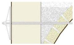
Fig. 22. Steel tie-rod in a barrel vault (Source: Caleca, 2018)
