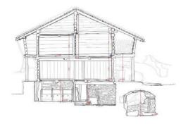
Fig. 3. Transversal section drawing of House 1. At lower floor, stables and the living room divided by a wooden partition; at first floor bedrooms; at the upper flow warehouses reachable by an external wooden (Drawing by Verona).
