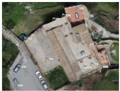
Fig. 7. Textured model of the villa in the software Agisoft Metashape, with the GCP used to link the two point clouds.
