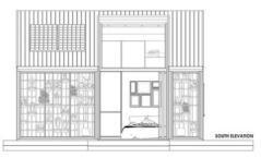
Fig. 3. The house south façade showing the integrated design of the hybrid Trombe wall and the green wall as passive systems.
