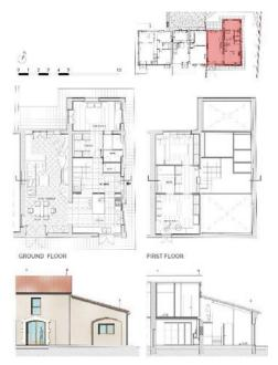
Fig. 4. The Unit 3 project: ground floor, first floor, main façade, longitudinal section. On the left side of the building: the barn. On the right, the peasant house. (Source: Li Puma, 2021)
