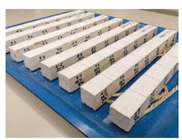
Fig. 2. Pieces of dimensions 290 x 25 x 25 mm
