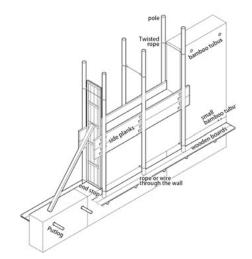
Fig.8 The formwork used in northern Fujian (author)
