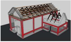
Fig. 4. Diagram of the reinforced concrete structure, in red, incorporated into the adobe walls in Uquia @ Authors
