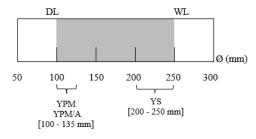
DL = dry limit; WL = wet limit; YPM = mechanically sprayed gypsum; YPM/A = lightened mechanical sprayed gypsum; YS = gypsum for traditional continuous pavements.
