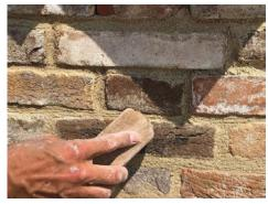
Fig. 6. Detail of a research experiment undertaken in collaboration between the Iuav, the Scuola Edile Padova, and a Venetian artisan to make and test the performances of traditional plaster and brickwork samples (Source: Squassina, 2021)
