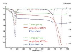
Fig. 3. Thermogravimetric analysis comparative for diverse types of gypsum
