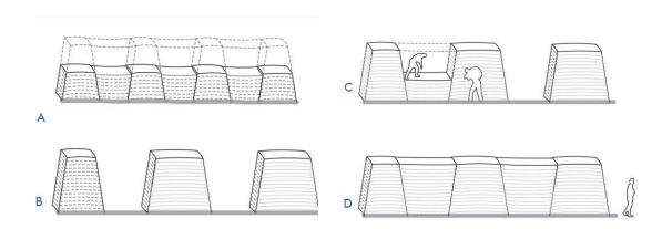
Fig. 4. A sequence of possibilities in the construction of segmental walls. A: Blocks built simultaneously. B, C, and D: Alternating construction (Source: Torres, 2021).
