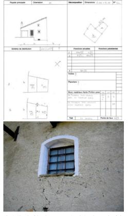
Fig. 9. Sketch of the plaster survey (Arvier) and example of plaster (Allein).
