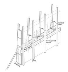
Fig.5 The integral formwork (author)
