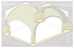
Fig. 16. Barrel vault with lunettes (Source: Caleca, 2018)
