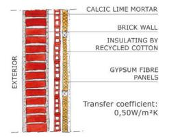
Fig. 5. Exterior brick walls details, section (Source: Li Puma, 2021)
