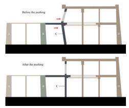
Fig. 9. Schematic view of the structural intervention concept. A - rebuilt porch (phase 1); B - tilted wall of the entrance with paintings; C - mixed structure on two storeys with paintings (phase 2); D - rest of the temple (phase 3).
