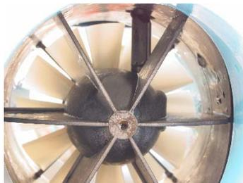
FIGURA 16. DETALLE DE LA PARTE INTERNA DEL CONTADOR WOLTMAN.
