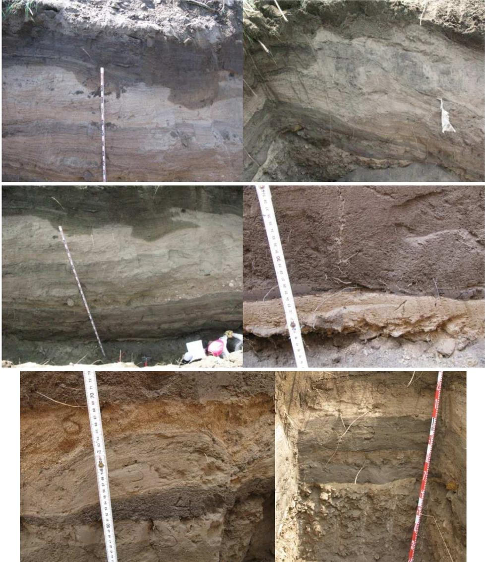
**Figure 2.9 – Laminated deposit behind a small check dam.**
