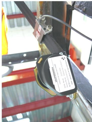
FIGURA 47. LOAD CELL EL20-16KN.
