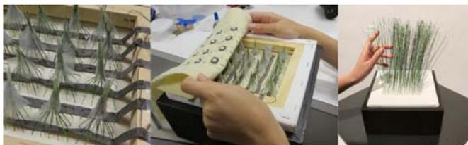
Fig. 3. Fiber optic bundles (left), LED matrix (middle), Light Pattern on Fiber optics (right)
