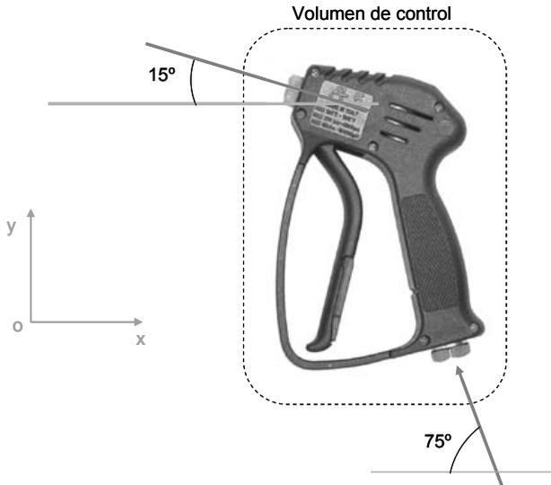
$$Q = 19 \text{ l/min} = 3,16 \cdot 10^{-4} \text{ m}^3/\text{s}$$
