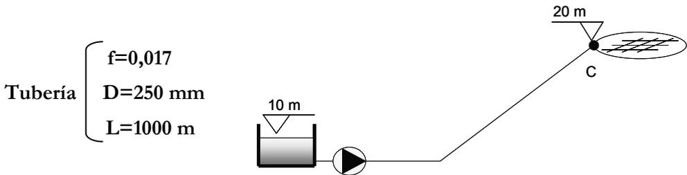
$$\left( \begin{array}{l} \text{B1: } h_B = 35-3500 \cdot Q^2 \quad Q \text{ en m}^3/\text{s} \\ \text{B2: } h_B = 48-3000 \cdot Q^2 \quad h_b \text{ en mca} \end{array} \right)$$
