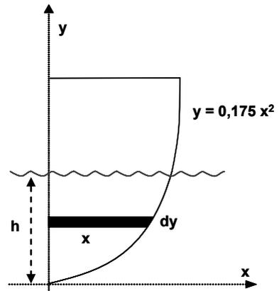
$$V_{\text{sumergido}} = 300 = 1,593 b^{3/2} \cdot 2 \cdot 30 \rightarrow b = 2,144 \, m$$
