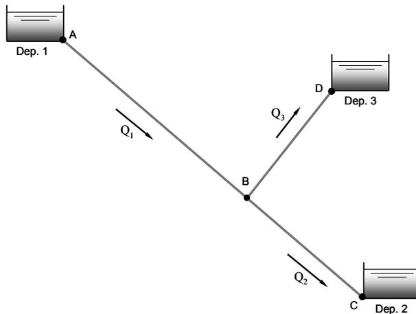
$$Z_1 = Z_2 + \frac{8f_{AB}L_{AB}}{\pi^2 g D_{AB}^5} Q_1^2 + \frac{8f_{BC}L_{BC}}{\pi^2 g D_{BC}^5} Q_2^2$$
