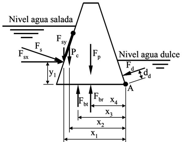
$$\begin{aligned} F_{sx} &= F_s \text{ sen } \alpha = \\ &= 10452990 \text{ sen } 78,69^\circ = \\ &= 10250000 \text{ Kp} \end{aligned}$$
