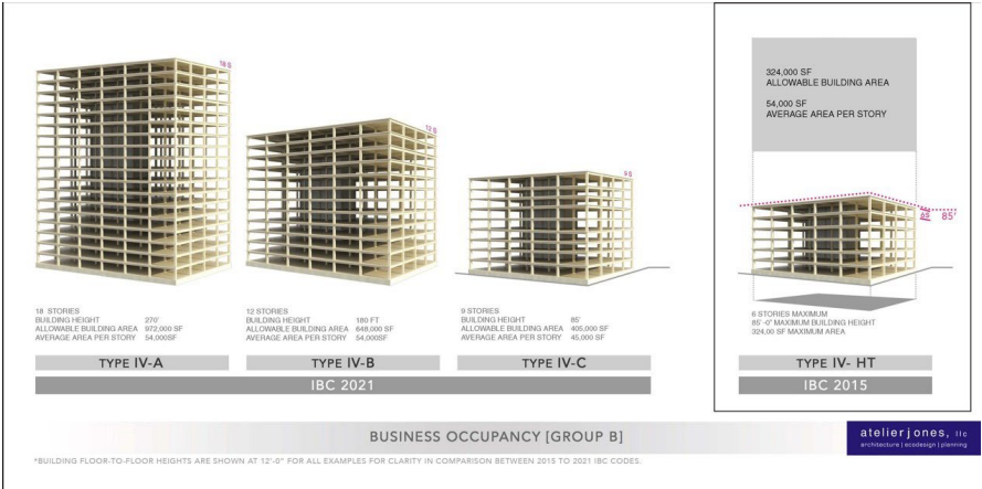
Figure 1. Mass Timber Code (IBC 2021). Source: (Atelier Jones, LLC n.d.). "CLT is a large-scale, prefabricated, solid engineered wood panel. Lightweight yet very strong, with superior acoustic, fire, seismic, and thermal performance, CLT is also fast and easy to install, generating almost no waste onsite. CLT offers design flexibility and low environmental impacts" (APA 2018).
