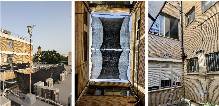
Figure 2. Location of the measurement instruments. a) weather station PCE-FWS 20, b) data loggers TESTO 174H, c) nebulizers at 2.00 m (6 seg/min)
