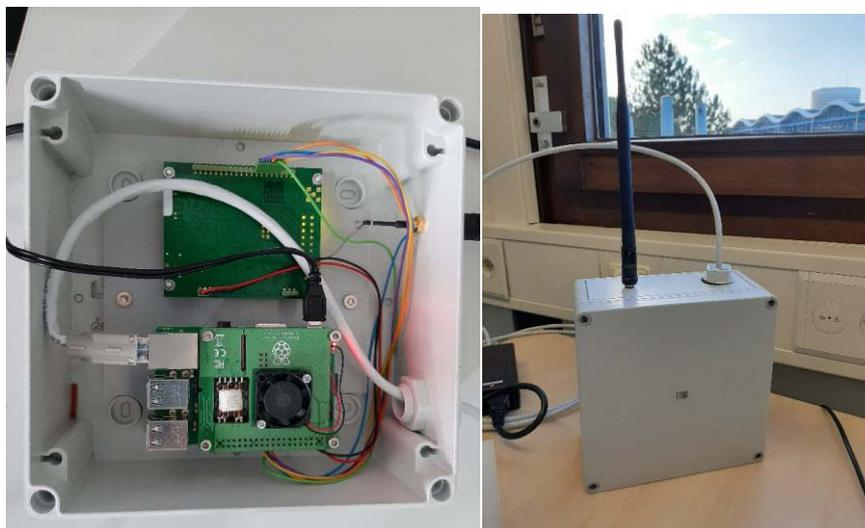
*Figure 2: Prototype of LoRaWAN Gateway*
