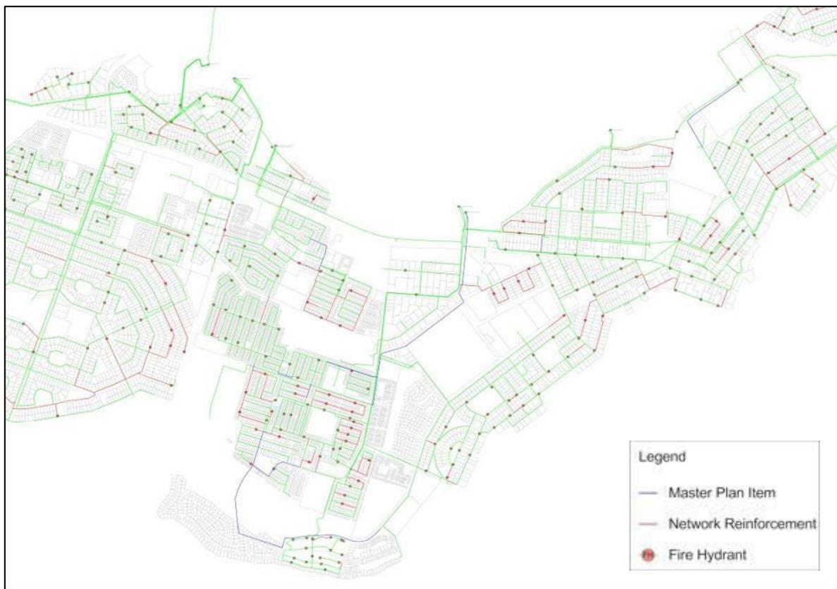
Figure 6. Test Case Network upgrades
