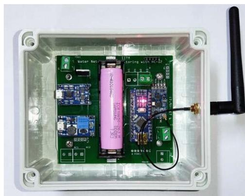
*Figure 2. Sensor interface module*
