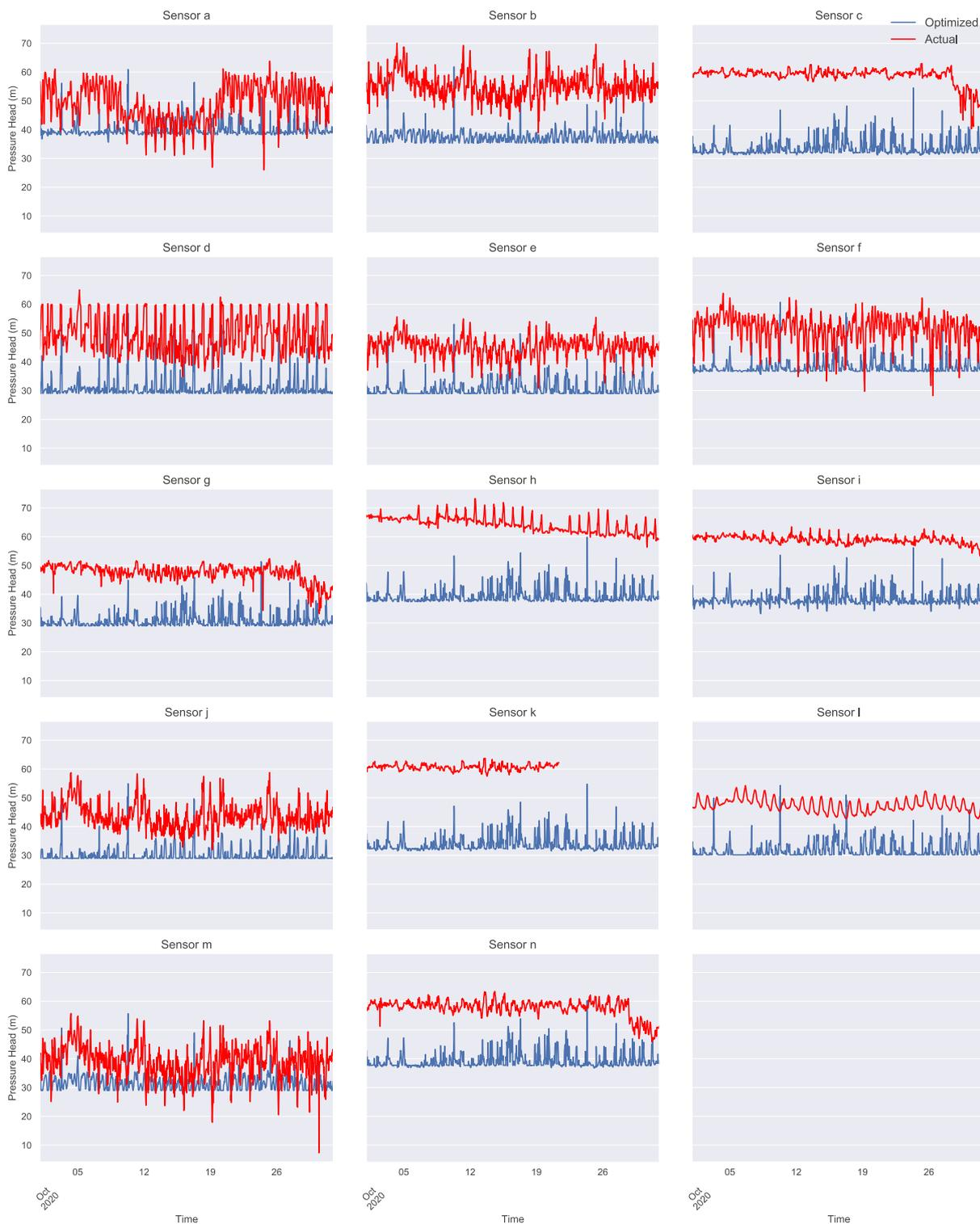
Figure 8. Comparison of optimized and actual pressure heads (m) at network junctions where pressure sensors are available. The optimization constraints at these junctions specify that pressures must be above 29 m (41 psi). The purpose of this plot is to illustrate how the levels of service in the form of pressure constraints are being applied and respected.
