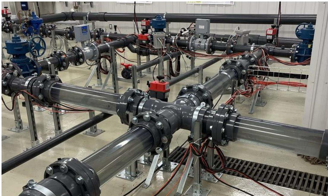
Figure 2. 150-mm cross junction used in mini water distribution network laboratory of INRS
