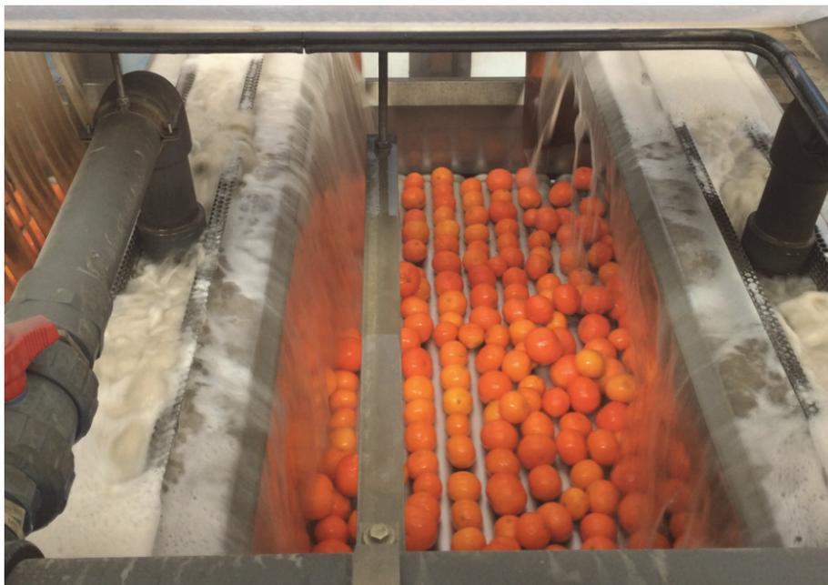
*Figura 13. Balsa catarata o drencher on-line.*
