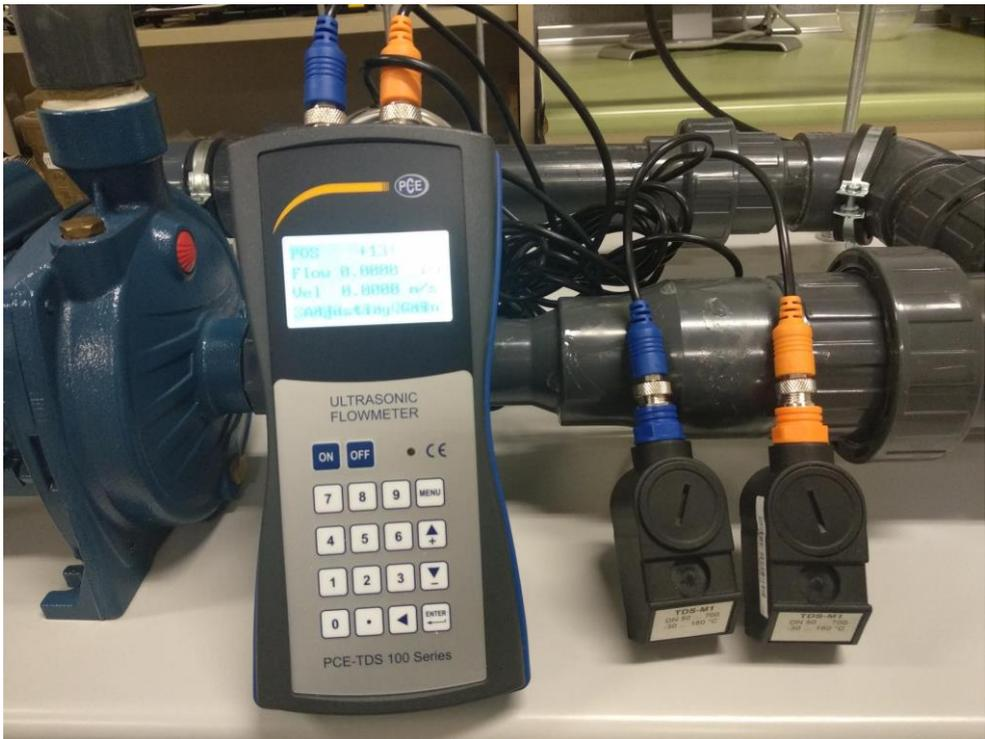
Figure 2. Ultrasound flow meter
