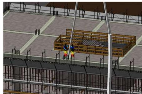
Fig 4 Modeling of the construction phase "casting with pump truck"
